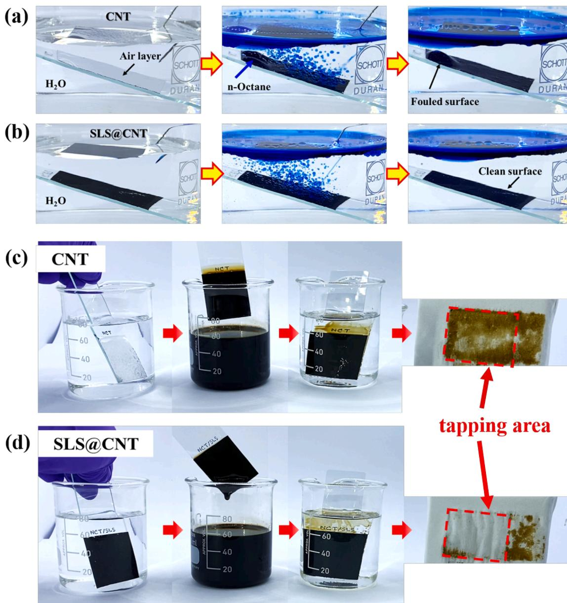
**Fig. 5.** Comparison of the antifouling and self-cleaning properties of the CNT and the SLS@CNT membranes. The (a) CNT and (b) SLS@CNT membranes were injected with isooctane underwater. The prewetted (c) CNT and (d) SLS@CNT membranes were immersed in crude oil, cleaned by water and tapped on tissue papers.
