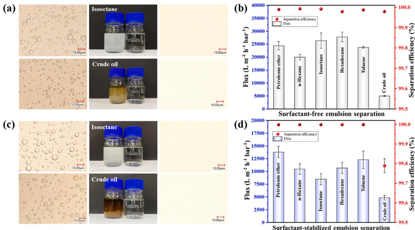
Fig. 6. (a) Actual images of isooctane and crude oil SFOWEs before and after filtration using the fabricated SLS@CNT membrane. (b) Separation performance against SFOWEs of the SLS@CNT membrane. (c) Actual images of isooctane and crude oil SSWEs before and after filtration using the SLS@CNT membrane. (d) Separation performance against SSWEs of the SLS@CNT membrane.
