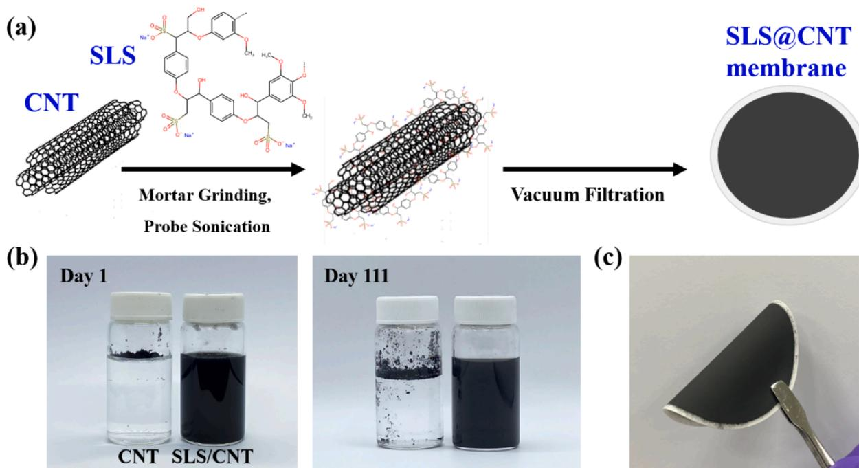
**Fig. 1.** (a) Schematic illustration of SLS@CNT membrane preparation. (b) Photographic images of CNT (left) and SLS@CNT (right) aqueous suspensions. The SLS/CNT aqueous suspension is stable for 3 months. (c) The SLS@CNT membrane exhibited good flexibility.
