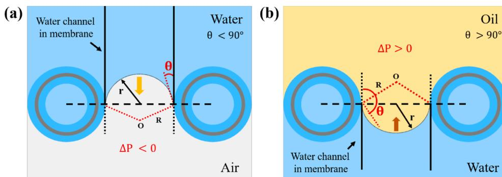
Fig. 8. Schematic diagram showing the wetting models of SLS@CNT membrane. (a) Water could permeate the SLS@CNT membrane. (b) Oil could not permeate the water-pretreated SLS@CNT membrane.
