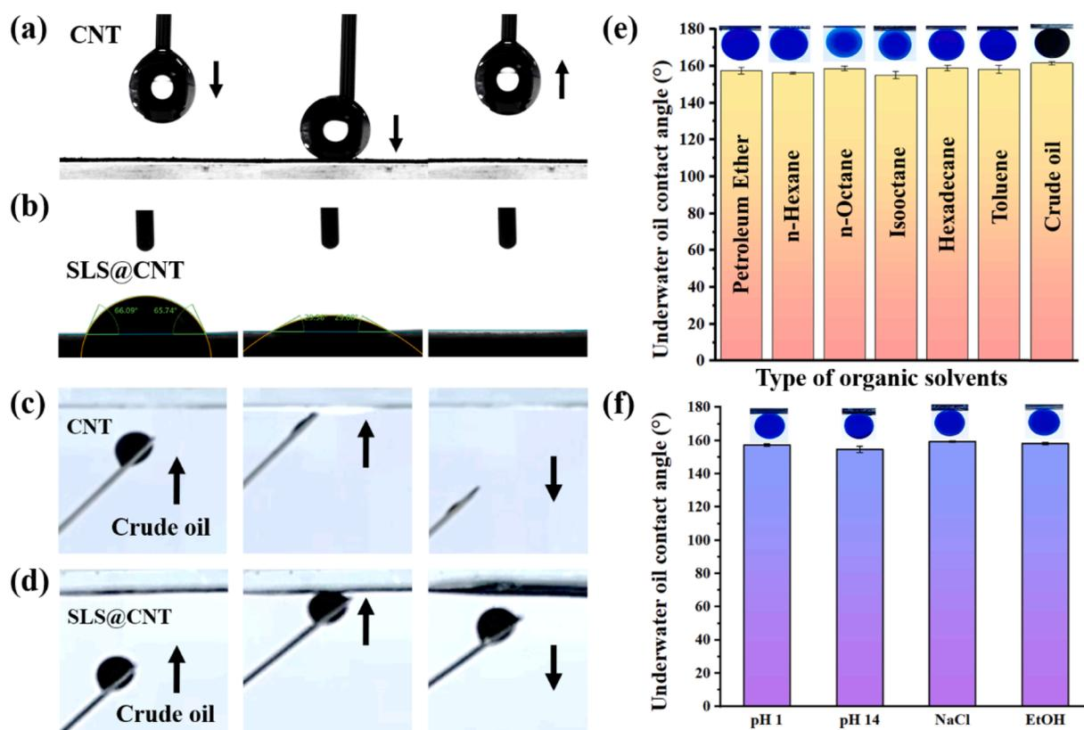
**Fig. 4.** Approach and contact of a water droplet in air on a syringe needle with respect to the (a) CNT and (b) SLS@CNT membranes. Approach, contact, deformation, and departure of a crude oil droplet underwater on a syringe needle with respect to the (c) CNT and (d) SLS@CNT membranes. (e) UWOCAs on the SLS@CNT membrane of a series of oils. (f) UWOCAs of SLS@CNT membranes after immersion in HCl (pH = 1), NaOH (pH = 14), NaCl (3.5 wt%) aqueous solutions, and ethanol for 7 days.
