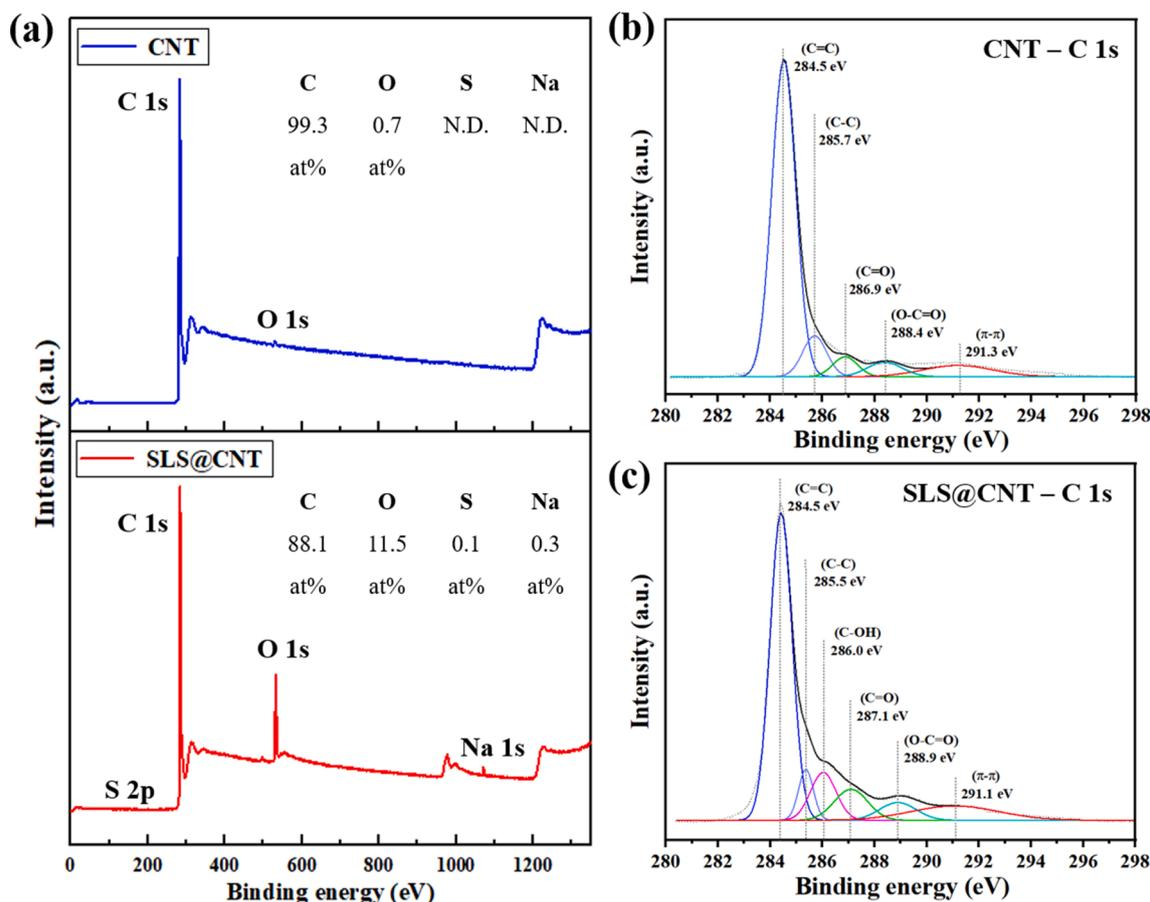
Fig. 3. (a) XPS spectra of the CNT and SLS@CNT membranes. High-resolution C 1s spectra of (b) CNT and (c) SLS@CNT membranes.
