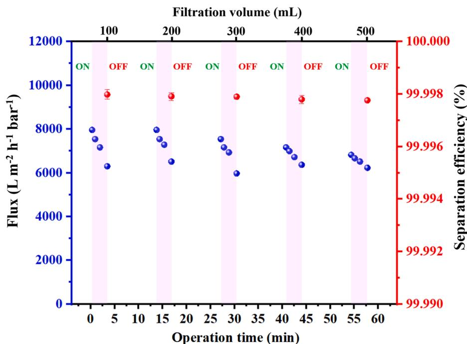
Fig. 7. SLS@CNT membrane's flux and separation efficiency during the separation cycles against SSWEs.
