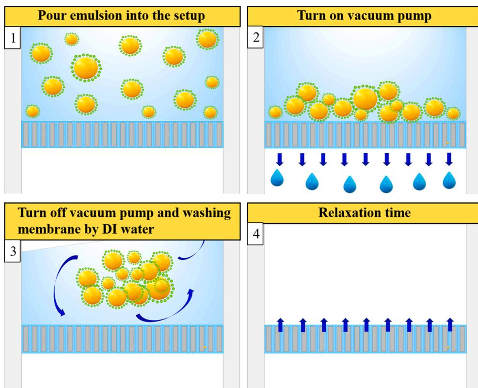
Fig. 9. Schematic diagram showing the emulsion separation and the self-cleaning mechanisms of the SLS@CNT membrane.
