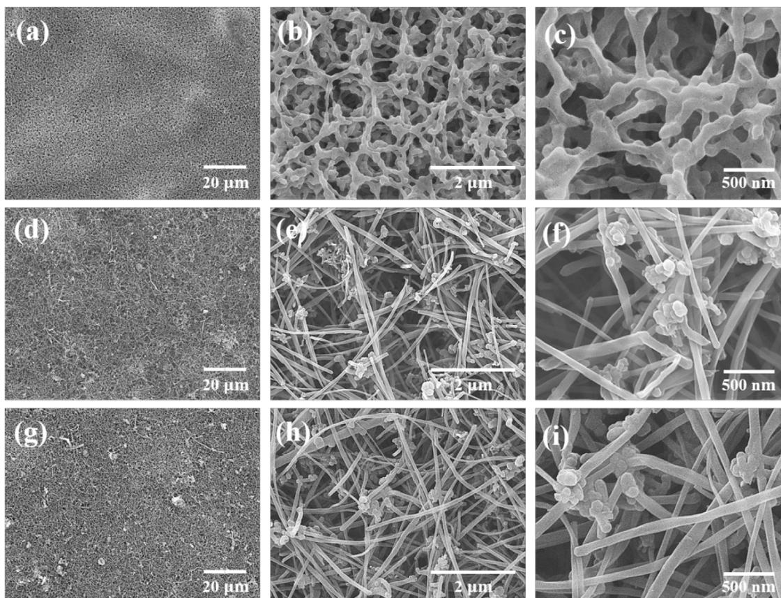
Fig. 2. The SEM images of (a-c) cellulose acetate substrate, (d-f) CNT membrane, and (g-i) SLS@CNT membrane with different magnifications.
