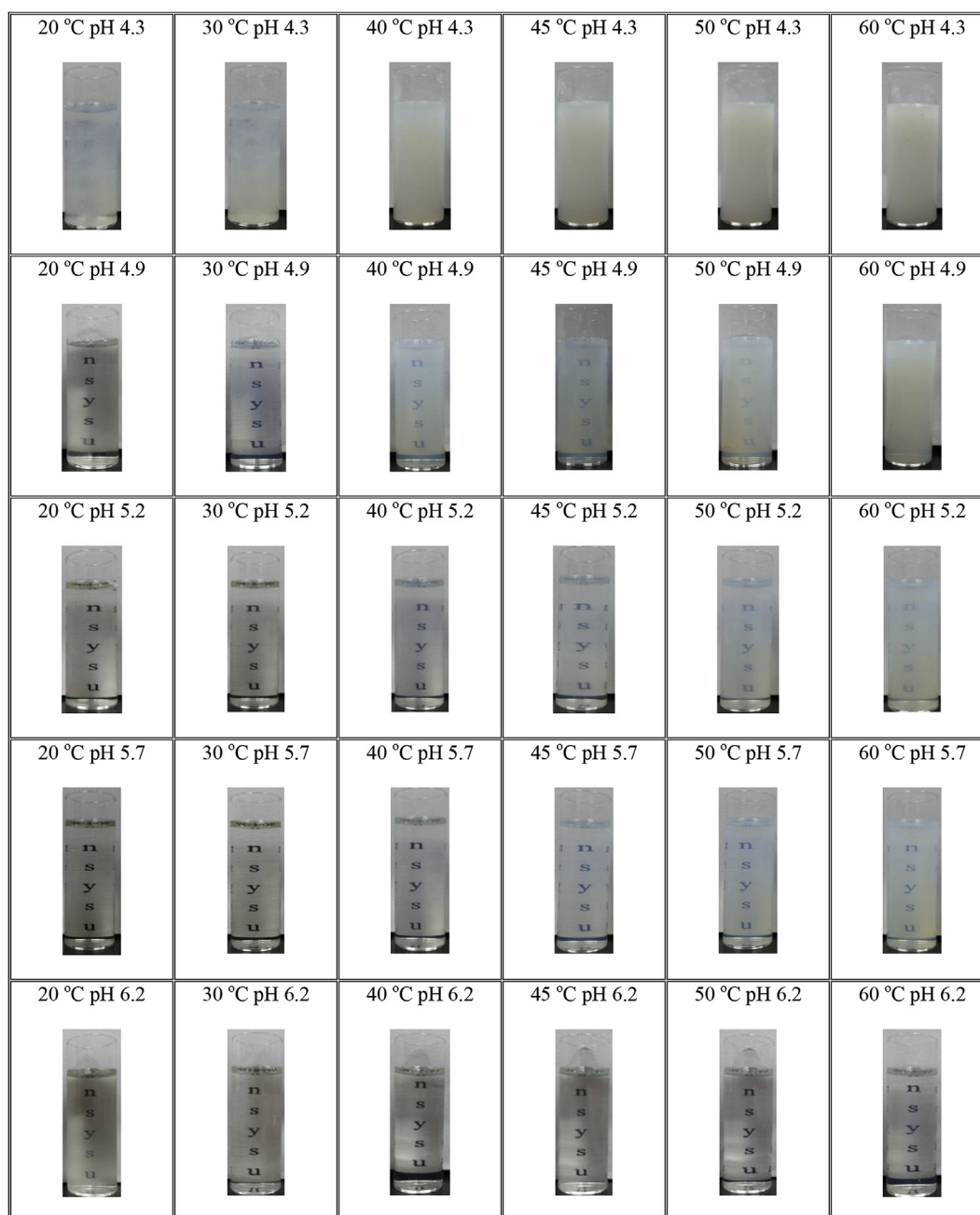
Fig. 10. Corresponding LCST behavior in photographs of the PNIPAm93- b -PMAA7 block copolymer in aqueous solution at various temperatures and values of pH.
