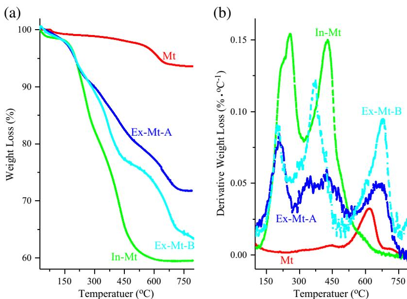
Fig. 2. (a) Weight loss and (b) derivative weight loss of Mt, In-Mt, Ex-Mt-A, and Ex-Mt-B.
